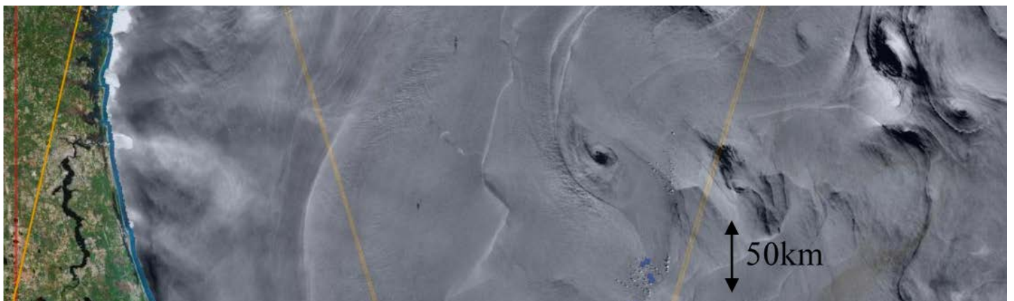
Satellite picture of sea surface roughness offshore of Florida. Sea surface roughness is modulated by the Gulf Stream and surrounding eddies.
